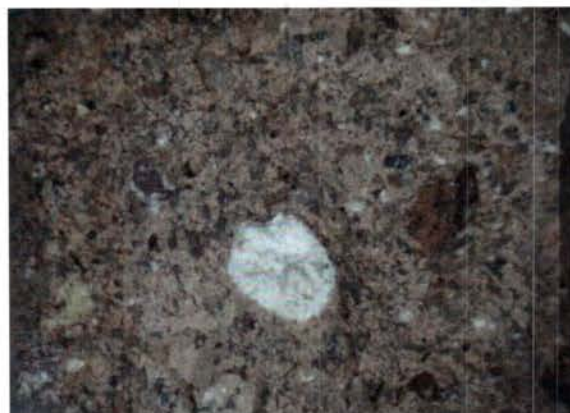
18 th century stone mortar – reddish brown sand suspended within a light reddish brown matrix, with lime nodules/blebs visible to the naked eye. Photomicrograph, 10x magnification in color-balanced light.
