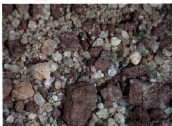
Sands extracted from 19 th century stone mortar. Photomicrograph, 10x magnification in color-balanced light.
