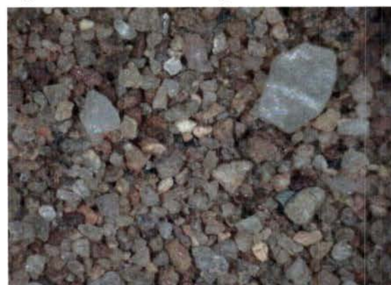
Sands extracted from 18 th century stone mortar. Photomicrograph, 10x magnification in color-balanced light.
